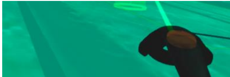
Figure 4.6 – Illustration of Teleportation Interaction Demonstrating the VR Controller and Selected Destination Marked by a Green Cylindrical Shape
