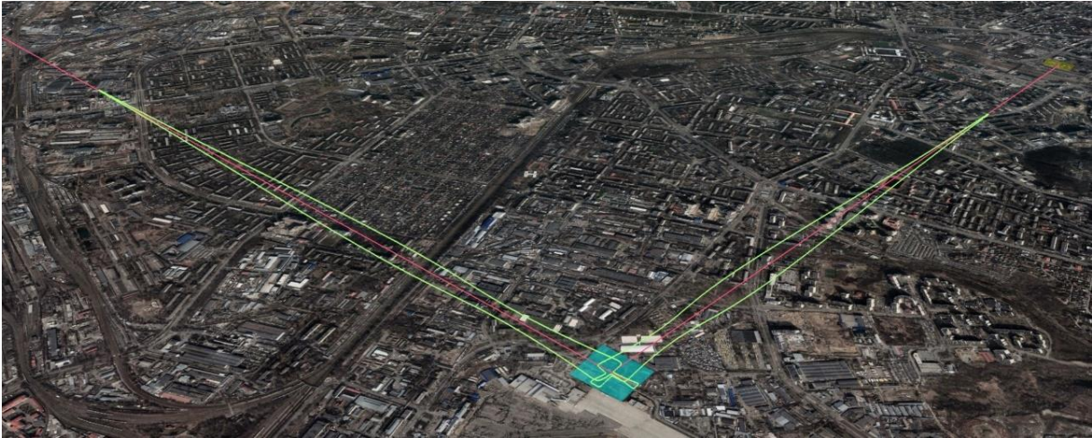
Fig. 3. Third-party risk levels for Scenarios 1 and 2: blue area - Vertiport area; the red line is the straight trajectory of the UAM aircraft (Track 1 and 2), light green – equal risk contour 10^{-6} , yellow circles are areas of multi-story buildings crossing the trajectory of the UAM aircraft.
