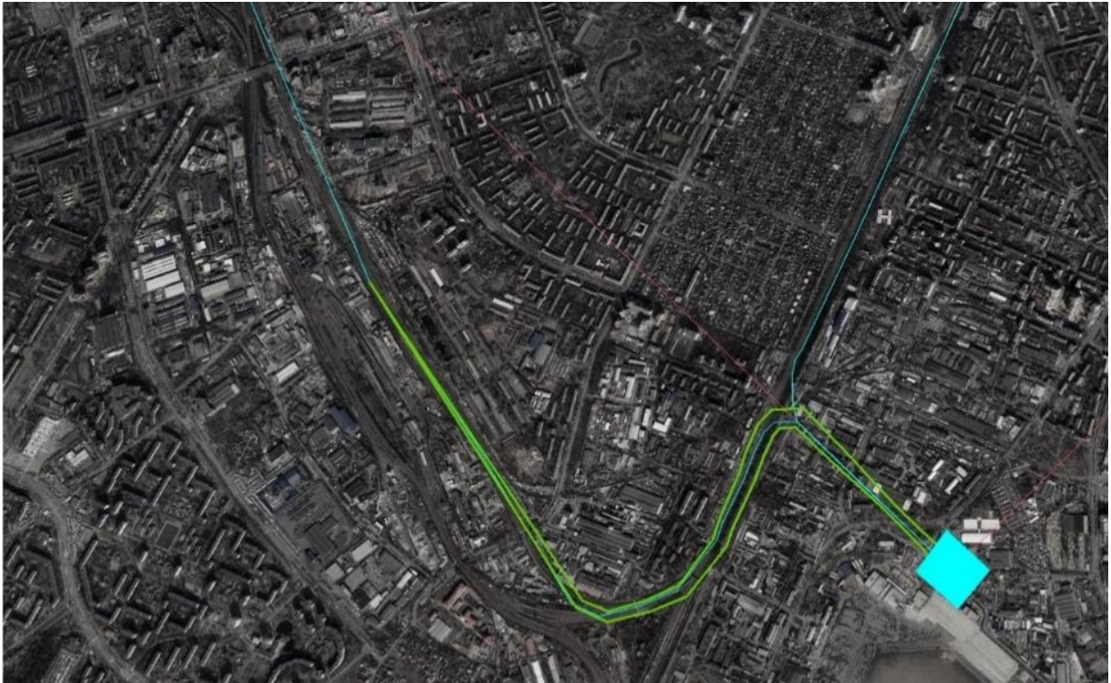
Fig. 4. Third-party risk levels for Optimized Scenario 3: blue area - Vertiport area; the red line is the straight trajectory of the UAM aircraft (Track 1X), light green – equal risk contour 10^{-6} , yellow circles are areas of multi-story buildings crossing the trajectory of the UAM aircraft.
