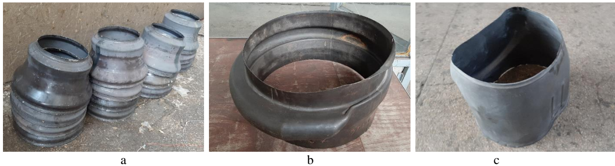
Fig. 6. Samples of parts obtained by explosive forming using an intelligent process optimization system: a – series of «Stator» parts; b – «Volute» («Cochlea») part; c – «Housing» part
