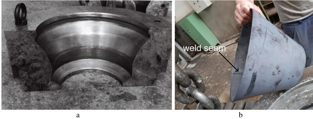
Fig. 3. Preparation for forming a «Stator housing» part: a – semi-die; b – workpiece
